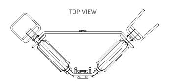
Note: Accessories shown are not included; X-Lab is required to be bolted to a concrete sub-floor
